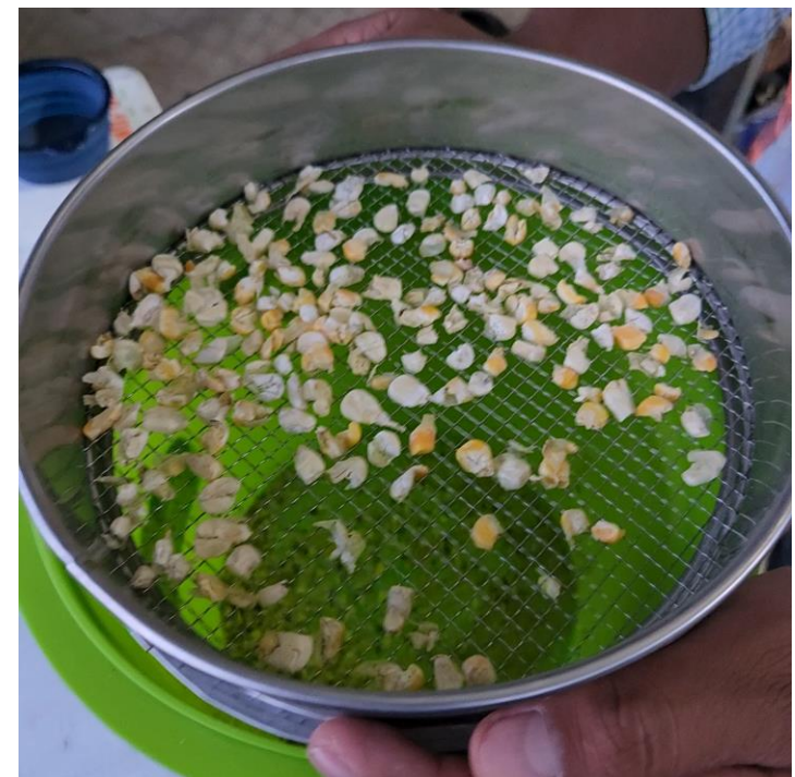
Run through sieve, 10 sec in each direction, 2X
