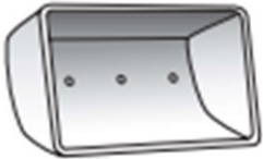
#1 VENT - Same holes in body as bolt mounting holes.
