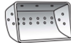
#4 VENT - Same as #3, plus three holes in each end cap.
