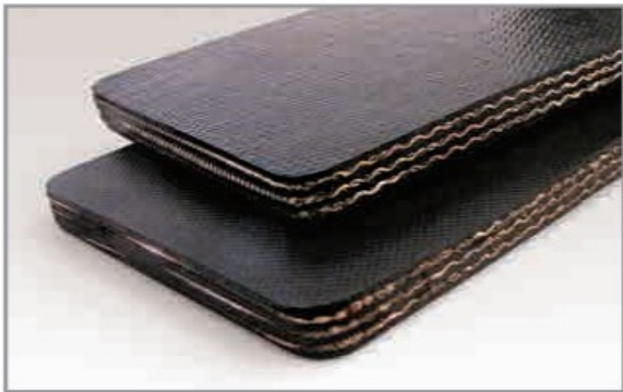
RUB 600 3 PLY, 1/16 x 1/16 SOR-SC-FR (EP1050/3 1.5 + 1.5 NBR)
