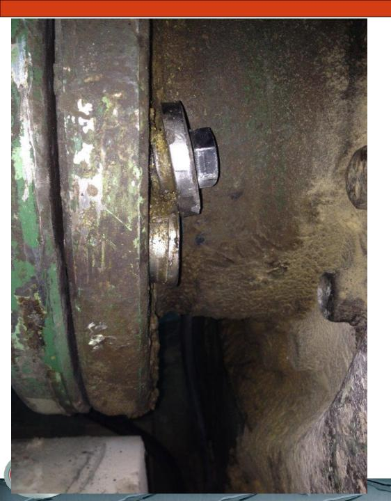
Shear Pin bushings coming out of shear pin housing (not correct)
